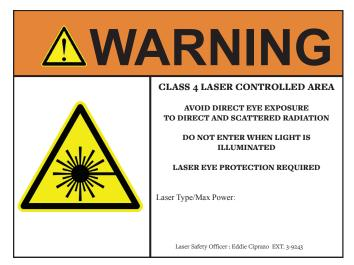
Standard laser WARNING sign for a Class 4 laser. Complete the blanks on the sign and post as directed by the LSO.
